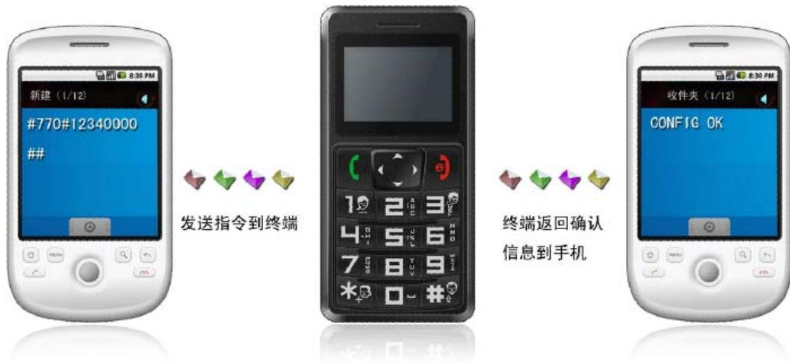
Send command to the terminal The terminal will return confirmation message to the mobile phone
