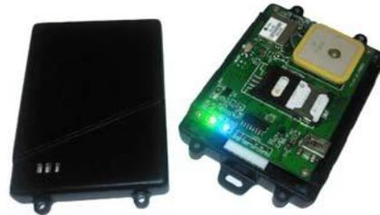
Find a suitable place on the motorcycle for installing the unit.,where the unit can get better GPS signal.Wiring connections must be firm and reliable and the joints should be wrapped with insulating tape tightly. The unused electrical wire should be properly insulated|
