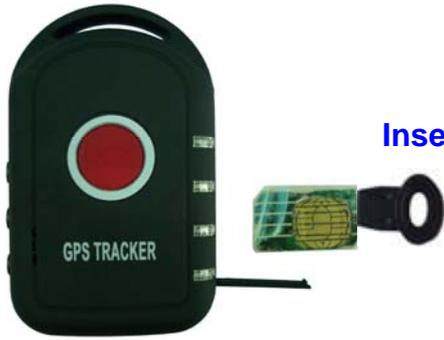
**Insert the sim card with the key**
